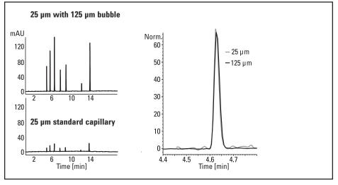
Analysis of cold medicine ingredients in a standard capillary (25 µm id) and an Agilent Extended Light Path Capillary
