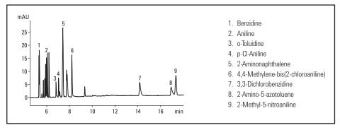
CZE analysis of basic amines using PVA coated capillaries (decomposition products of azo dyes)
