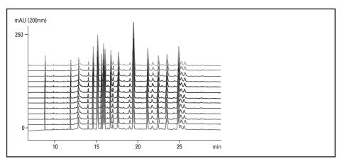
CZE of a tryptic digest of recombinant human growth hormone using a standard fused-silica capillary with 75  $\mu m$  internal diameter
