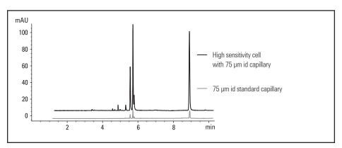
Agilent high sensitivity detection cell vs. 75 µm standard capillary for the CZE separation of naphthalene sulfonic acids
