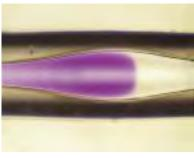
Electroosmotic flow maintains the "plug" flow in the bubble. Optical slits matched to the zone geometry maintain resolution.
