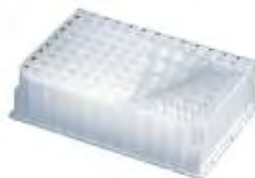
Collection plate, showing 96-position closing mat, 5042-1389
