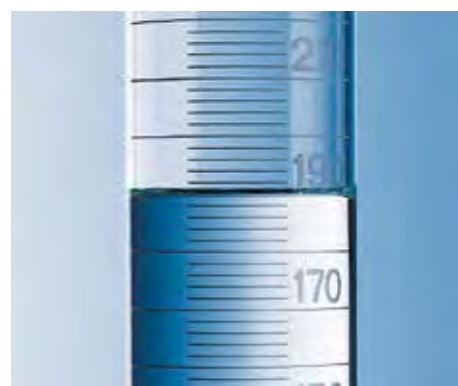
SILBERBRAND. Short graduation marks. Reading at lowest point of meniscus.
