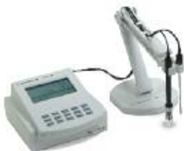
3200P standard pH meter, G4383A
