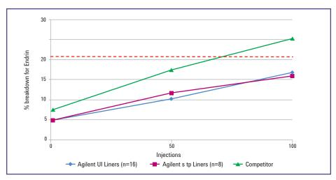
Agilent Ultra Inert Liners with wool are superior vs. the competition as shown in this endrin breakdown comparison.
