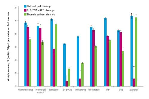
EMR—Lipid significantly removes matrix contributions, improving recovery across many analytes and minimizing your need for separate workup and methods.
