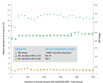
With EMR—Lipid there is less need for system maintenance and calibration due to fewer sample matrix interferences. As a result, fewer samples need to be re-run. This advantage lets you operate at higher throughput, resulting in cost savings and a more efficient lab.
