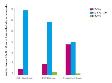
Higher efficiency matrix removal with EMR—Lipid results in higher precision and greater accuracy in results.
