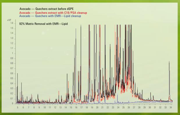
Figure 1. GC/MS full-scan chromatogram overlay of an untreated QuEChERS avocado extract (black), compared to traditional C18/PSA cleanup (red) and an extract treated with Agilent Enhanced Matrix Removal—Lipid (blue).
