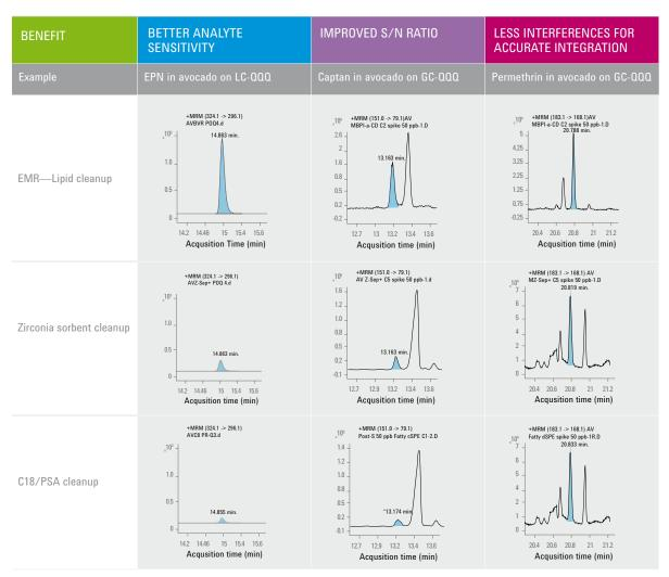
Figure 5. Improvements in chromatography can be seen in the analysis of samples prepared with Agilent Enhanced Matrix Removal—Lipid, including better sensitivity due to reduced matrix ion suppression, better signal-to-noise ratio, and fewer interferences providing accurate integration with GC or LC triple quadrupole systems.
