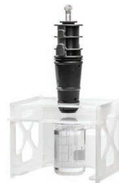
Torch cleaning stand, for 5100/5110 ICP-OES torches, G8010-68021
