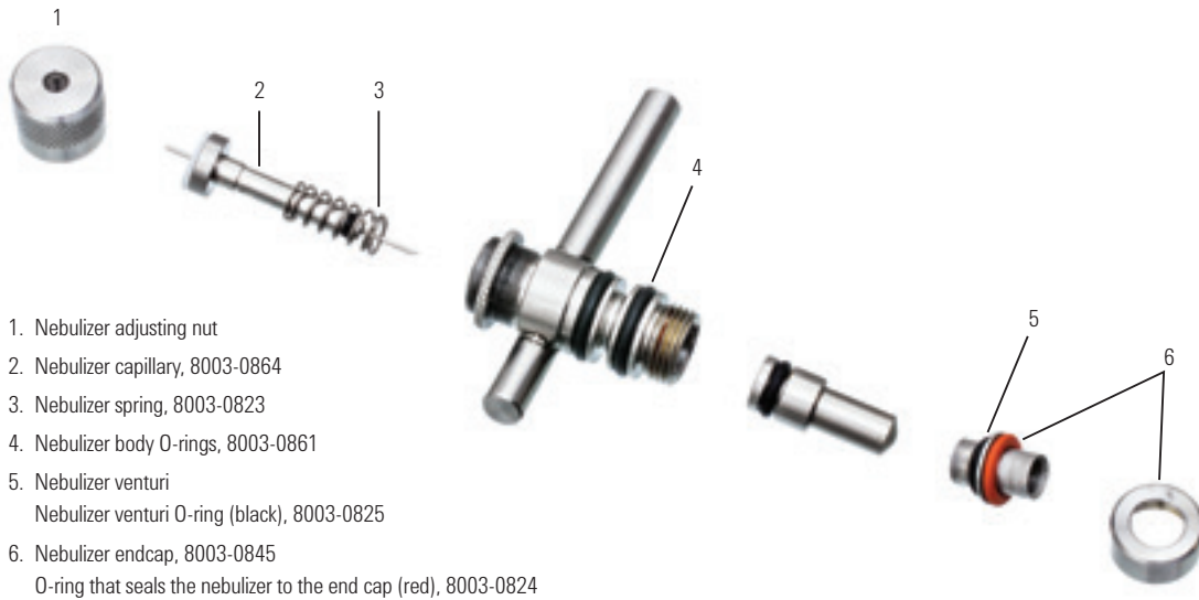
Exploded view of Nebulizer assembly, 8003-0828
